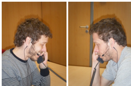
Figure 1. Identical twin pair in separate quite rooms holding a telephone conversation (task one) and recorded with flat-frequency response omnidirectional ear-mounted microphones.
