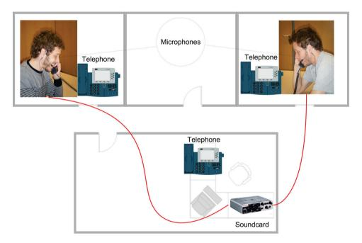
Fig. 1. Data collection set-up
