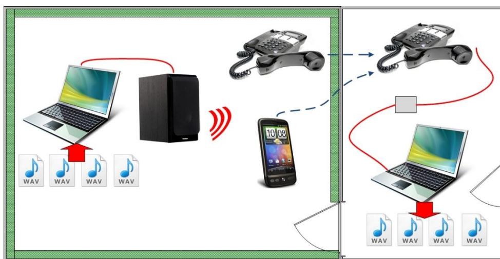
Figure 9. Set-up for the filtering of the audio signal.
